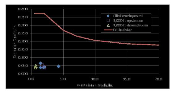
Effective corrosion rates based on the reported metal loss depth and age of Line 401 was determined. The apparent corrosion rate was relatively uniform across several
