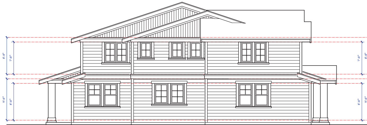
UNIT 1 NORTH ELEVATION DUPLEX A 1/4" = 1'-0"
