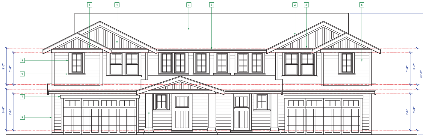
UNITS 1 & 2 WEST ELEVATION DUPLEX A 1/4" = 1'-0"
