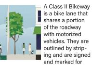
exclusive use by bicycle travel, providing service for one-way bicycle travel. Class II Bikeways are located next to the through lane for motorized vehicles.
