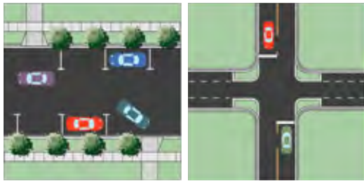
On-street Parking Bulb-out Intersection (intersection of Summit Drive and a Neighborhood Street)
