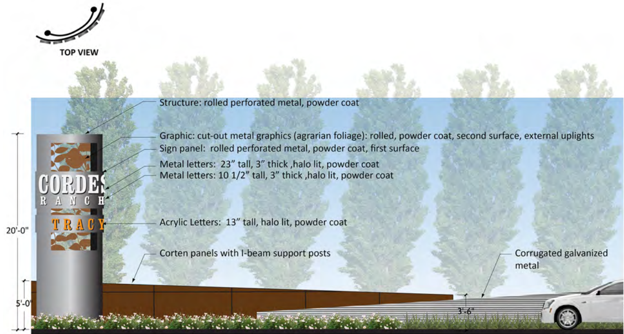
Figure 5.14, Project Entry Sign and Walls
