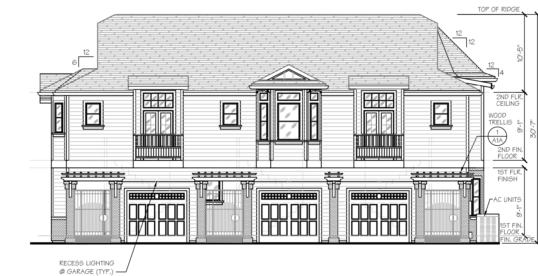
REAR MULTI FAMILY DWELLING UNIT ELEVATION SCALE: 1/8"=1'-0"
