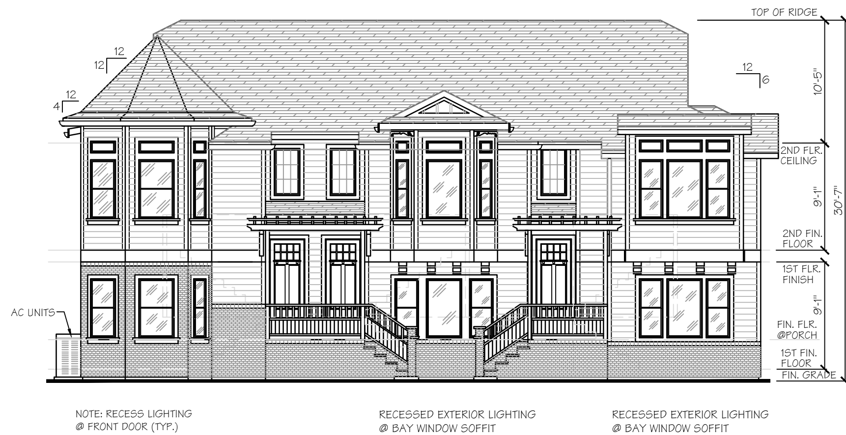
FRONT MULTI FAMILY DWELLING UNIT ELEVATION SCALE: 1/8"=1'-0"
