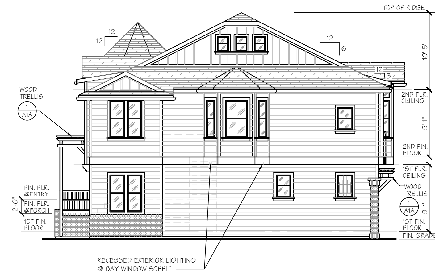
SIDE MULTI FAMILY DWELLING UNIT ELEVATION SCALE: 1/8"=1'-0"
