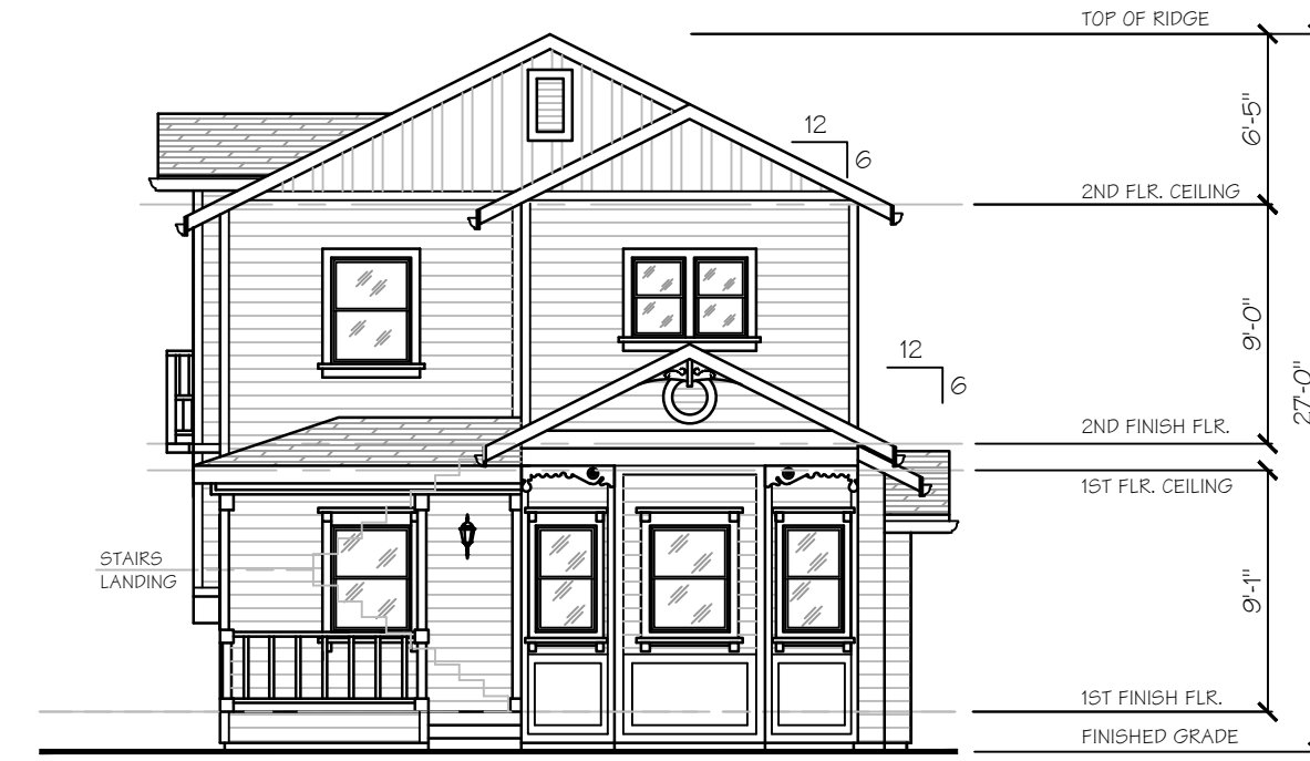
FRONT SINGLE FAMILY DWELLING ELEVATION RESIDENCE 1 & 2 SCALE: 1/8"=1'-0"
