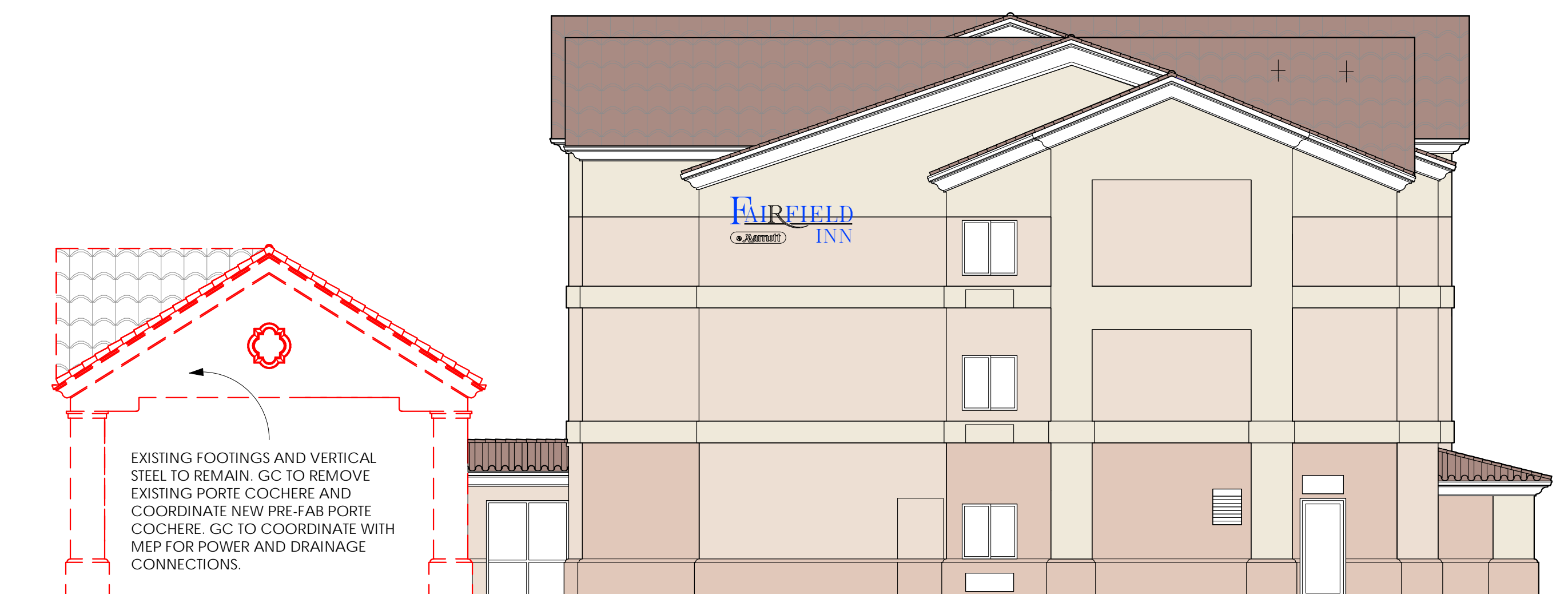
3 SOUTH ELEVATION - EXISTING AE-050 SCALE: 1/8" = 1'-0"
