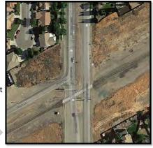
**Description**: Widening from a 4-lane arterial to a 6-lane major arterial which includes modification of existing 40' median to
