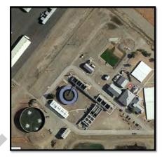
Description: The Upflow clarifier is an important componet of the water treatment process. Coagulation, floculation and
